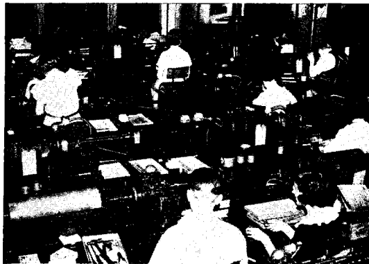
Grid Winding—Another delicate and accurate step in National Union tube making conducted under close expert supervision.
